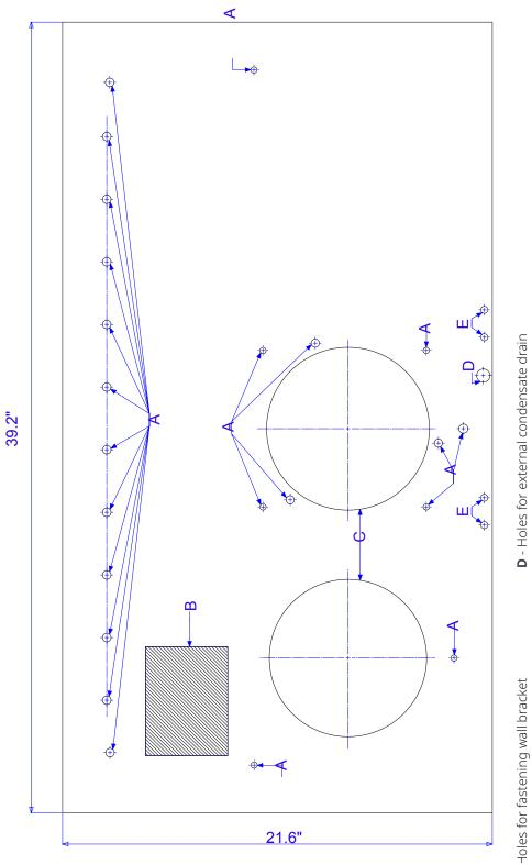
**D** - Holes for external condensate drain
